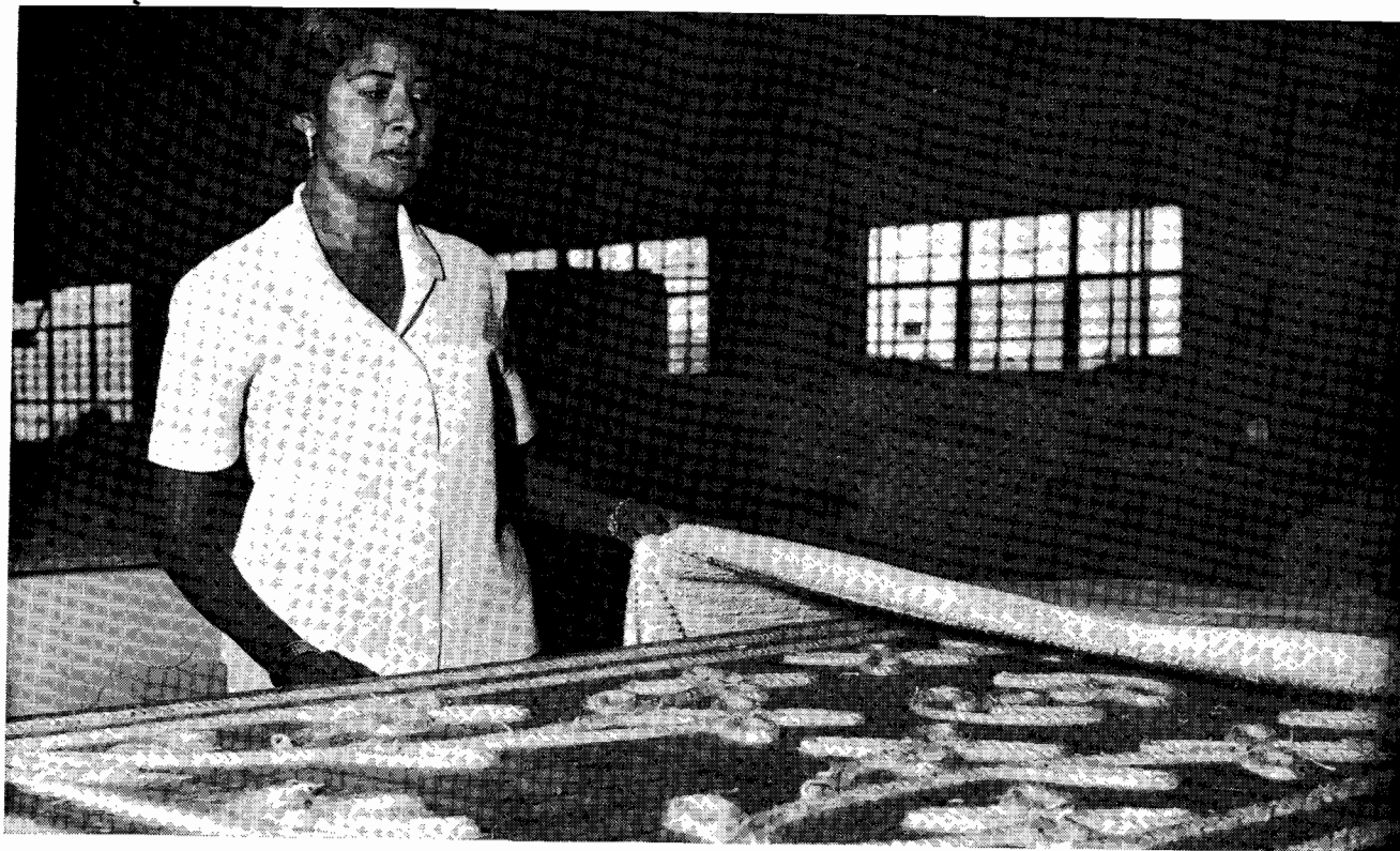
(Above): An ingenious method is used to mark the pattern on the candlewick cloth. Lengths of thin rope are laid out on a table according to the pattern and the bedspread is laid over them. Then the pattern is traced through the bedspread with a piece of chalk.
